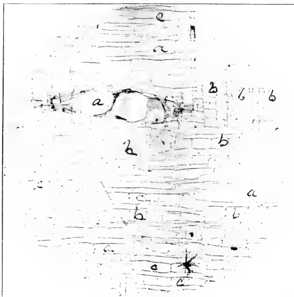
FIG. 3.—RADIAL SECTION, BALSA, ABOUT 70 DIAMETERS, SHOWING (a) LARGE VESSELS OR DUCTS, (b) MEDULLARY RAYS, (c) LONGITUDINAL CELL STRUCTURE.
